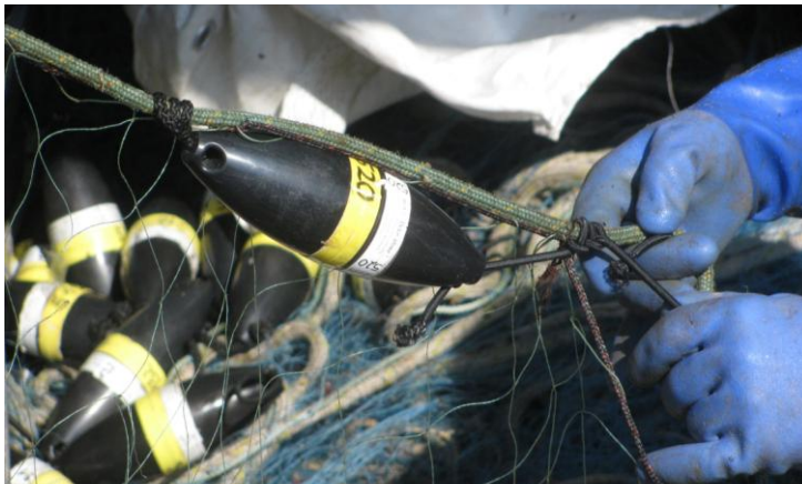
Fig. 3: PALfi attached to gillnet floatline.
